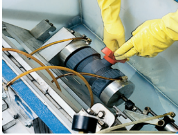
Colonial Full Block TUBVs are tested under high pressure for structural integrity and low pressure for a bubble-tight seal.
