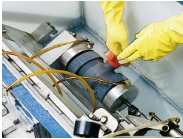
Colonial Single Union Ball Valves are tested under high pressure for structural integrity and low pressure for a bubble-tight seal.
