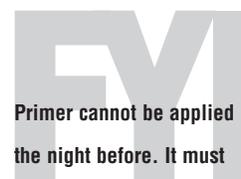
Primer cannot be applied the night before. It must be wet when cement is applied over the top of it.
